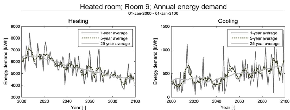
FIG 6. Annual energy demands for heating and cooling in a heated room
