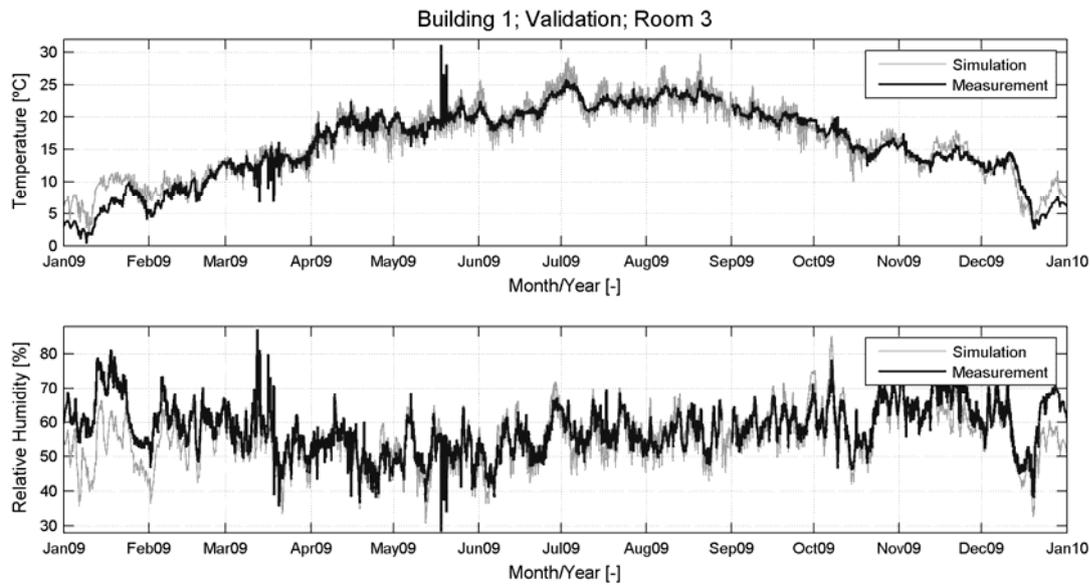
FIG 1. Validation of indoor climate simulation model
