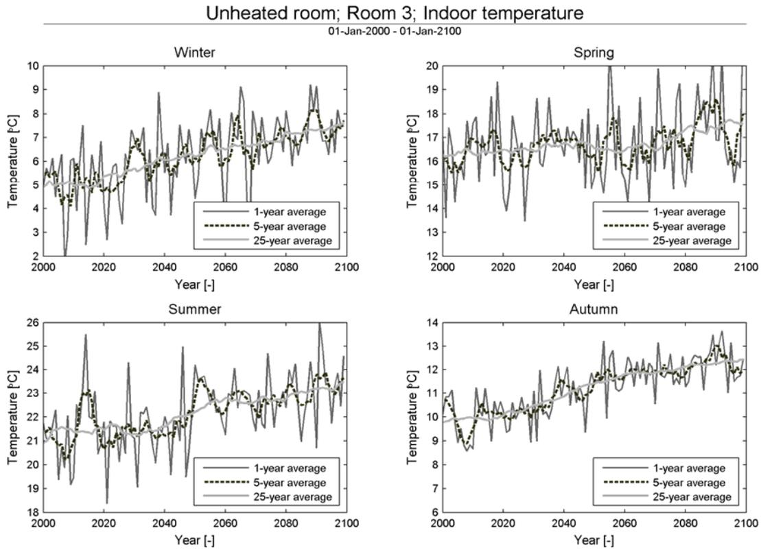
FIG 2. Indoor temperature in an unheated room, values averaged over periods of 1, 5 and 25 years
